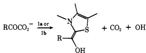
unit. We employed a Radiometer pH-stat (pH meter equipped with automatic titrator, autoburet, titrigraph recorder, and circulating temperature bath) to measure the rate of hydroxide ion release, where  $\text{R} = \text{CH}_3$  or  $\text{C}_6\text{H}_5$ . The initial velocity of these curves of  $\text{H}_3\text{O}^+$  consumed vs. time reflect the zero-order decarboxylation rates in the thiazolium-catalyzed model reactions, as the proton is consumed at the time of  $\text{CO}_2$  loss.
