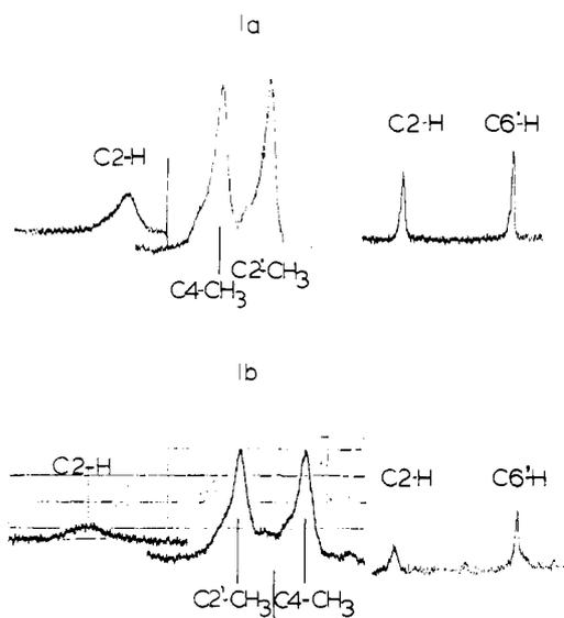
Figure 3. <sup>1</sup>H NMR line broadening studies in H<sub>2</sub>O at 60 MHz, pH 8.17 ± 0.02, 0.25 M concentrations of Ia and Ib, identical spectral parameters. Right-hand peaks in normal scan, left-hand peaks show expanded spectrum used for line width measurements. Primed positions pertain to the pyrimidine ring, unprimed to the thiazolium.
