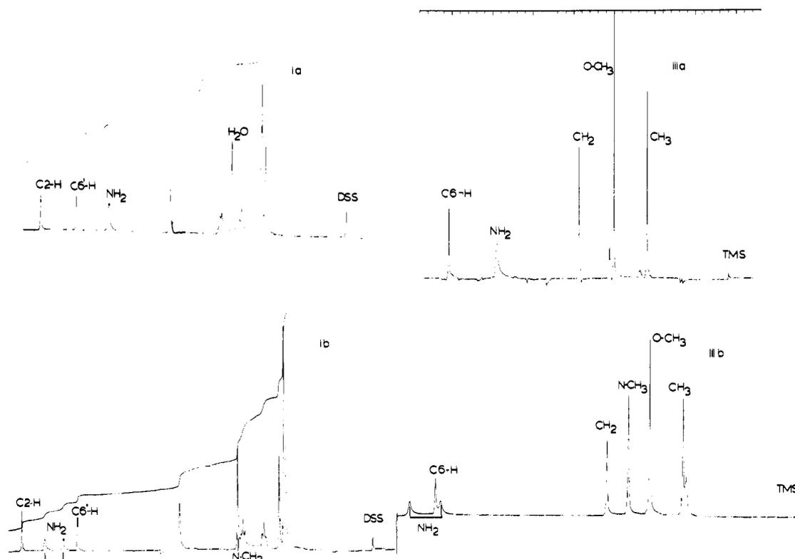
Figure 1.  $^1\text{H}$  NMR spectra in  $\text{Me}_2\text{SO}-d_6$ . Ia, Ib, and IIIa recorded at 1250 Hz, IIIb at 1000 Hz spectral width. Chemical shifts are listed in Table 1. The peaks near 2.5 ppm were complicated by residual  $^1\text{H}$  in the solvent.
