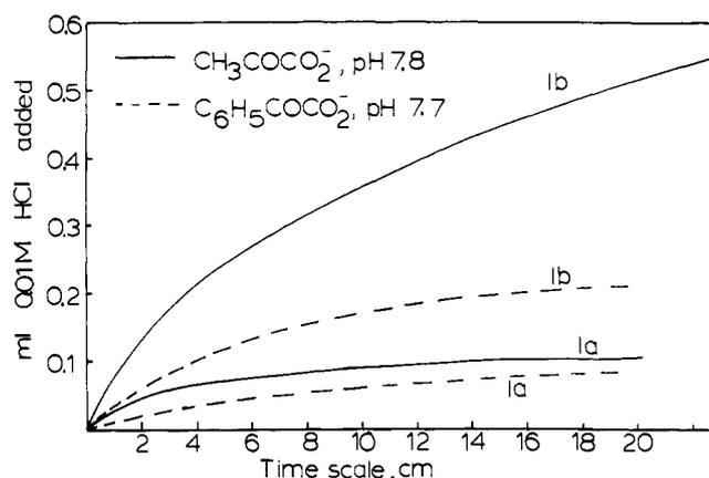
Figure 4. pH-Stat kinetic plots for decarboxylation of pyruvic and phenylglyoxylic acids. Chart speed for pyruvic acid, 2 min/cm; for phenylglyoxylic acid, 1 min/cm, 30 °C.
