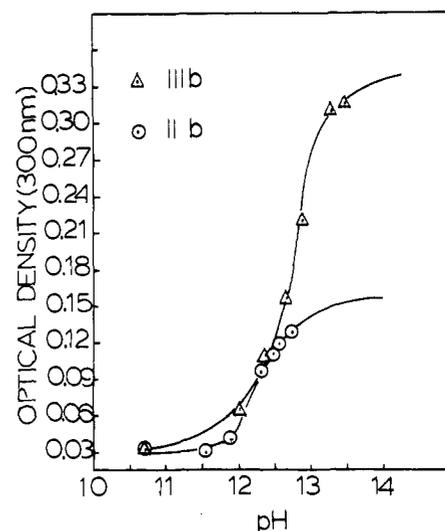
Figure 2. Ultraviolet *pK<sub>a</sub>* titration of IIb and IIIb.
